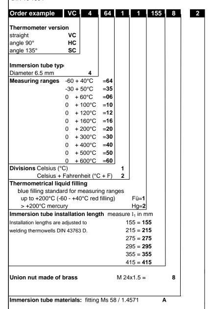
We deliver the thermometers of the type series "4" generally with a steel tube diameter 6.5 mm on the capillary lower part, suitable in thermowells with orifice 7 mm to protect the glass and to avoid that glass parts fall into the orifice of the welding cover when the capillaries break.
